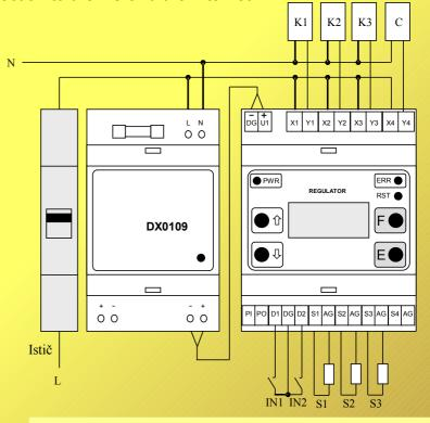
K1, K2, K3 – switches, C – pump IN1 – HI tariff, IN2 – attenuation, S1, S2, S3 – temperature sensors
