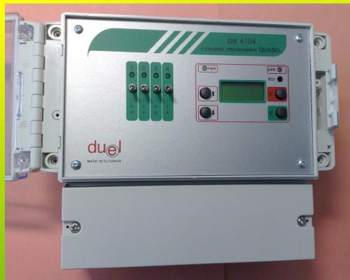
The device is a 4-channel programmable timer designed for year-round programming ringing of church bells.
