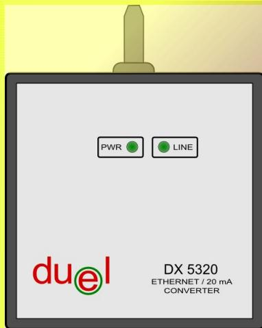
Converter DX5320 is designed to transmit the current loop condition via ethernet network to a computer, that emulates a virtual serial port.
