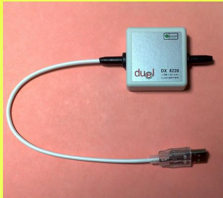
DX5220 converter is designed to convert conditions of the current loop signals to USB standart, the use for today's PCs.
