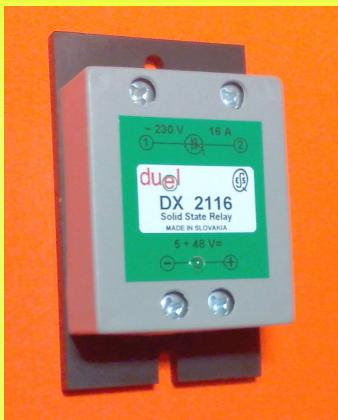
Contactless power switch DX2116 is an electronic relay, allowing switching of electric power. AC supply circuit 230V through a one-input control circuit which provides the shortcircuit switching element to the amount of time for the switch to the input terminals of the DC input is fed the control signal. This may be in the range of 5 to 48 V direct current. The control circuit provides switching the load connected when crossing the zero level of the supply voltage.
