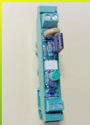
Contactless power switch DX2003 is an electronic relay, allowing switching of electric power. AC supply circuit 230V through a one-input control circuit which provides the shortcircuit switching element to the amount of time for the switch to the input terminals of the DC input is fed the control signal. This may be in the range of 5 to 48 V direct current. The control circuit provides switching the load connected when crossing the zero level of the supply voltage.
